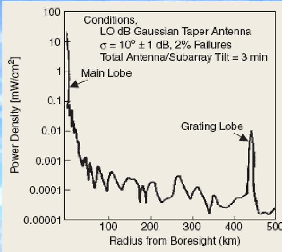
Predicted ground-level microwave power density for a full-power GEO SPS as a function of distance - Credit: J. M. Osepchuk, IEEE Microwave, "How Safe Are Microwaves and Solar Power from Space", *IEEE Microwave magazine*, vol. 3, issue 4, page 58-64, Dec. 2002.
